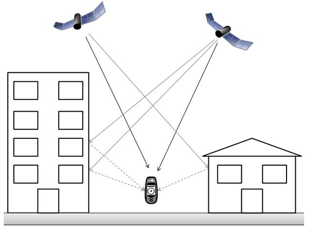
Fig. 6. Interference caused by reflection of the signals
