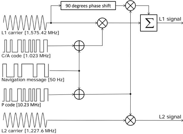
Fig. 2. Pilot signals and codes
