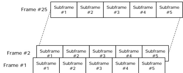
Fig. 4. GPS navigation message: masterframe structure.
