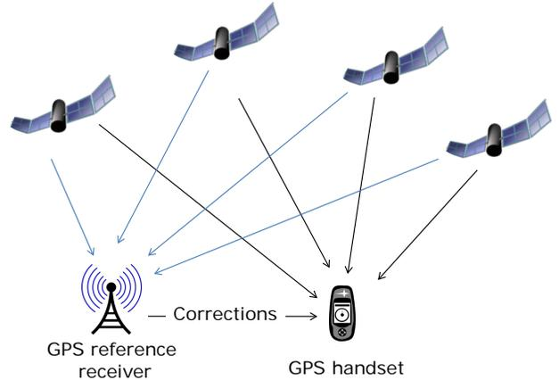
Fig. 8. Differential-GPS architecture
