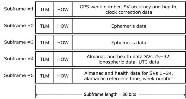
Fig. 3. GPS navigation message: frame structure
