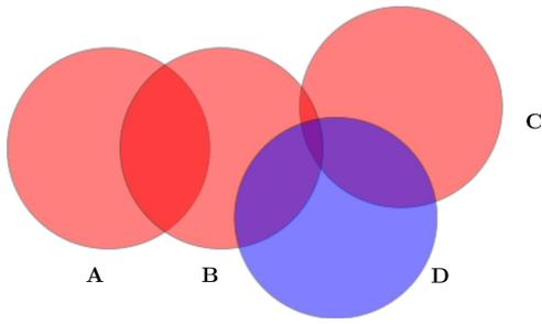
Fig. 1. Four femto cells next to each other, three of them using the same channel, causing interference.
