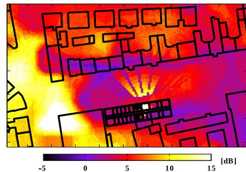
Fig. 2. The setup for signal strength measuring of a femto cell in a complex building from [3]
