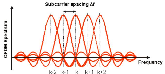
Figure 1. OFDM Spectrum [5]
