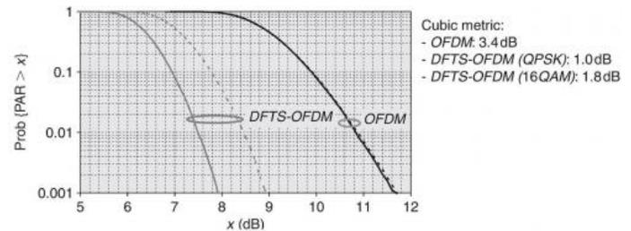
Figure 3. PAR distribution and cubic metric of OFDM and SC-FDMA (DFTS-OFDM), Solid curve: QPSK. Dashed curve: 16QAM [10]
