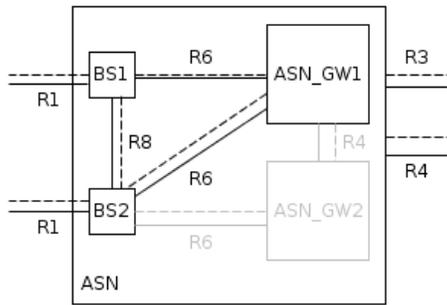
Figure 6. Reference Model of ASN decomposed in BS and ASN GW entities [16]
