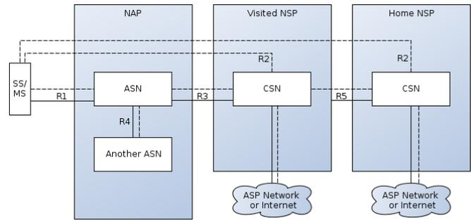
Figure 5. WiMAX Network Reference Model, adapted from [16], [17], solid lines: data bearer plane; dashed lines: control plane
