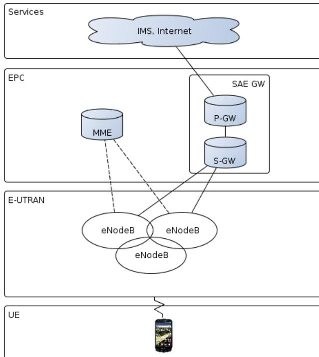
Figure 4. LTE System Architecture for E-UTRAN only, adapted from [11]
