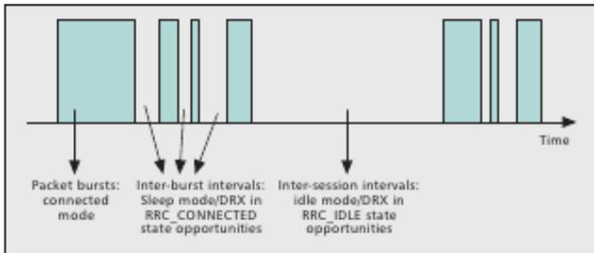
Figure 7. Mapping of power management modes to a generic traffic model [27]
