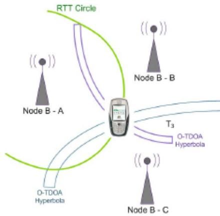
Fig. 9. The principle of OTDOA
