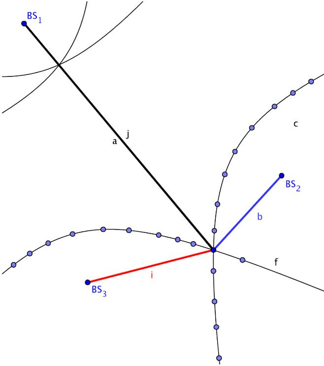
Fig. 6. TDoA - The intersection of the hyperbola  $c$  with the hyperbola  $f$  is the assumed position of the MS
