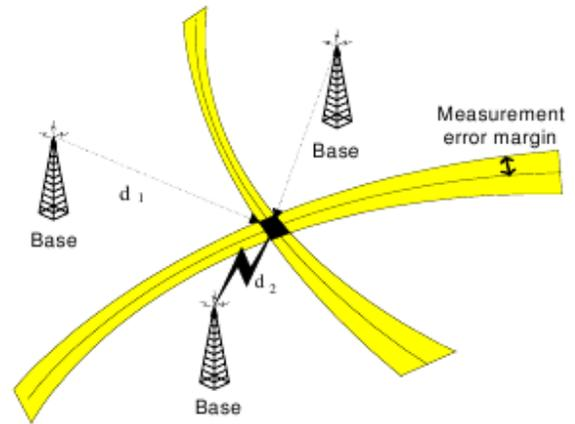
Fig. 8. The principle of E-OTD [13]
