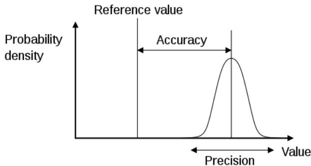
Fig. 14. Difference between accuracy and precision [wikipedia]
