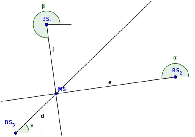
Fig. 4. AoA- The intersection of the lines from the BS in direction of the Angle of Arrival is the assumed position of the MS
