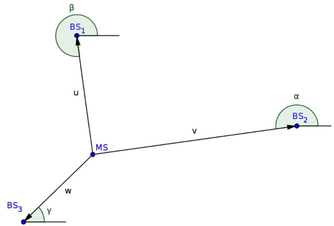
Fig. 3. AoA - The MS sends out a signal that is received by the antenna arrays from the BS
