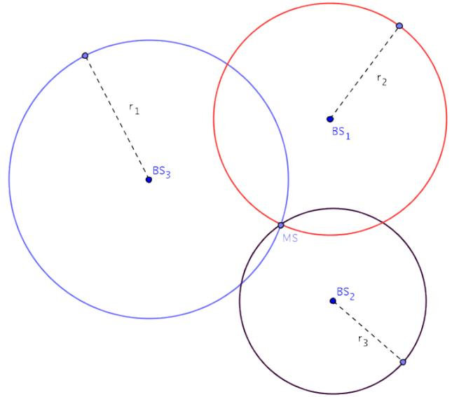
Fig. 5. ToA for the 2D case. Here 3 BS are enough to get an unambiguous position for the MS
