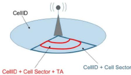
Fig. 2. The principle of Cell ID [4]
