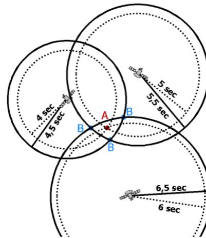
Fig. 10. 2D positioning with 3 satellites and adjustment of the clock error [19]
