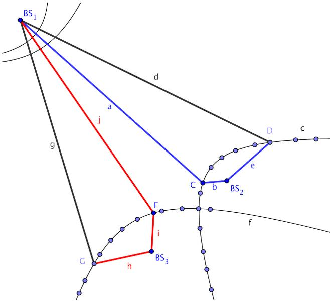
Fig. 7. TDoA - Two hyperbolas which represent possible points of residence for the MS.  $D, C, F, G$  are four such points with the correspond distances from the BS.
