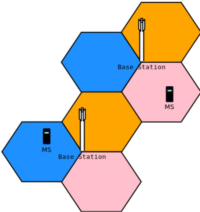
Fig. 1. CellID - Two Base Tranceiver Stations (BTS) with sectorized antennas
