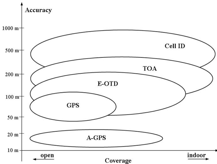
Figure 10. Coordinate System of different location techniques and their accuracies [5]
