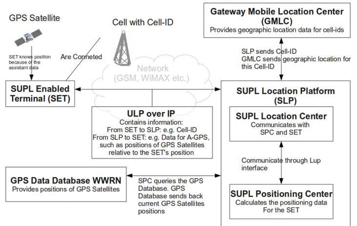
Figure 13. Example SUPL Architecture for A-GPS positioning with Cell-ID aid
