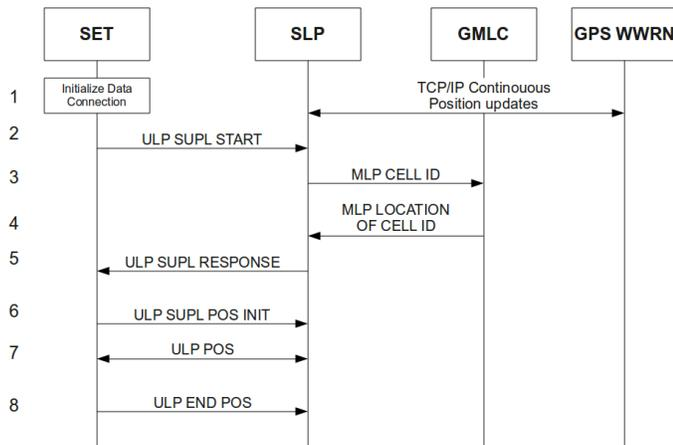
Figure 14. Set initiated A-GPS positioning sequence diagram, see also [15], [12] and [17]
