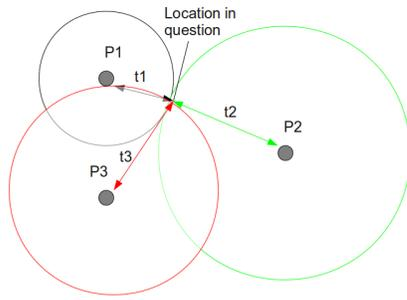
Figure 1. Trilateration example.  $t_1$ ,  $t_2$  and  $t_3$  are the different signal-run times and strengths which can be used to determine the location in question.
