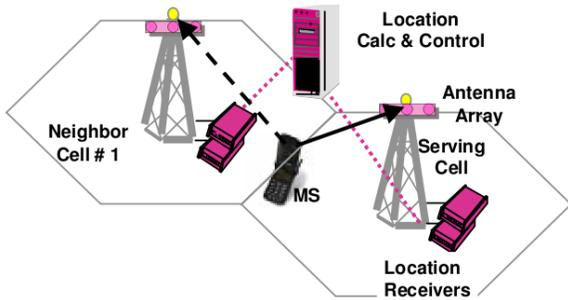
Figure 7. Angle of Arrival example for GSM [7]
